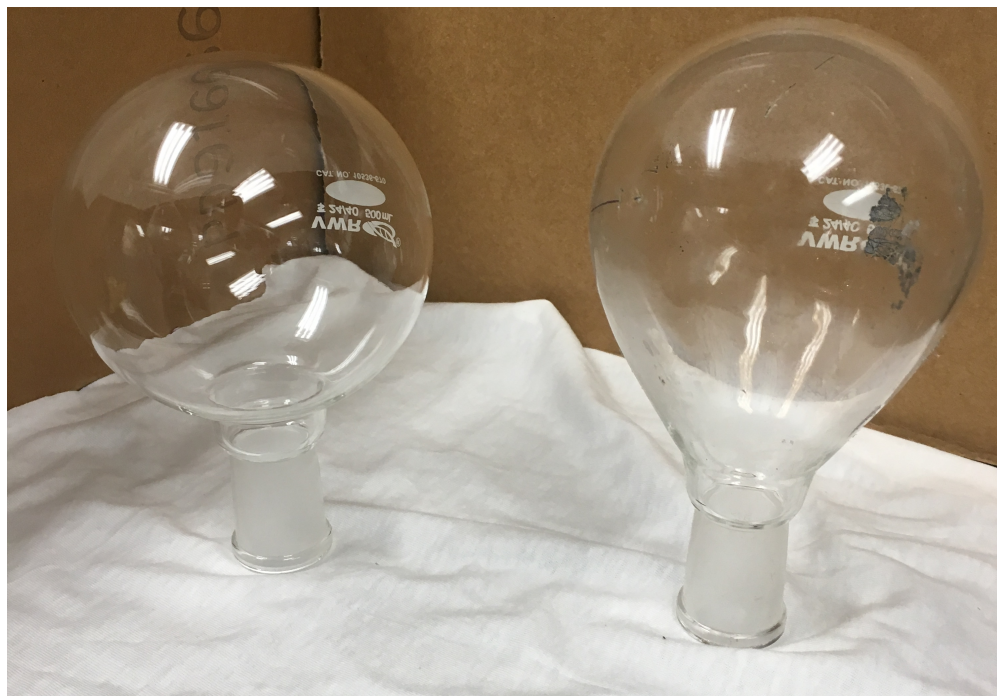
Figure 2.9: (left) Unused spherical flask and (right) Deformation of flask observed for T > 600^{\circ}\text{C} .
