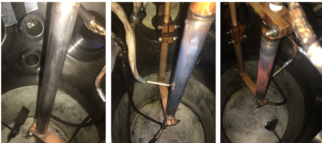
Figure 3.5: Comparison of the surface conditions observed in these experiments. (left) Polished stainless steel (middle) Typical oxide layer built up on surface after being held for 5-10 mins above 1000 K in an air atmosphere and (right) Surface after approximately 5 hydrogen ignition tests.
