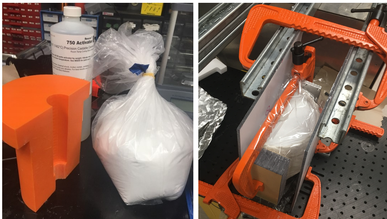
Figure 2.2: (left) Casting compound and 3D printed model of insulating holder (right) Ceramic curing in clay mold.
