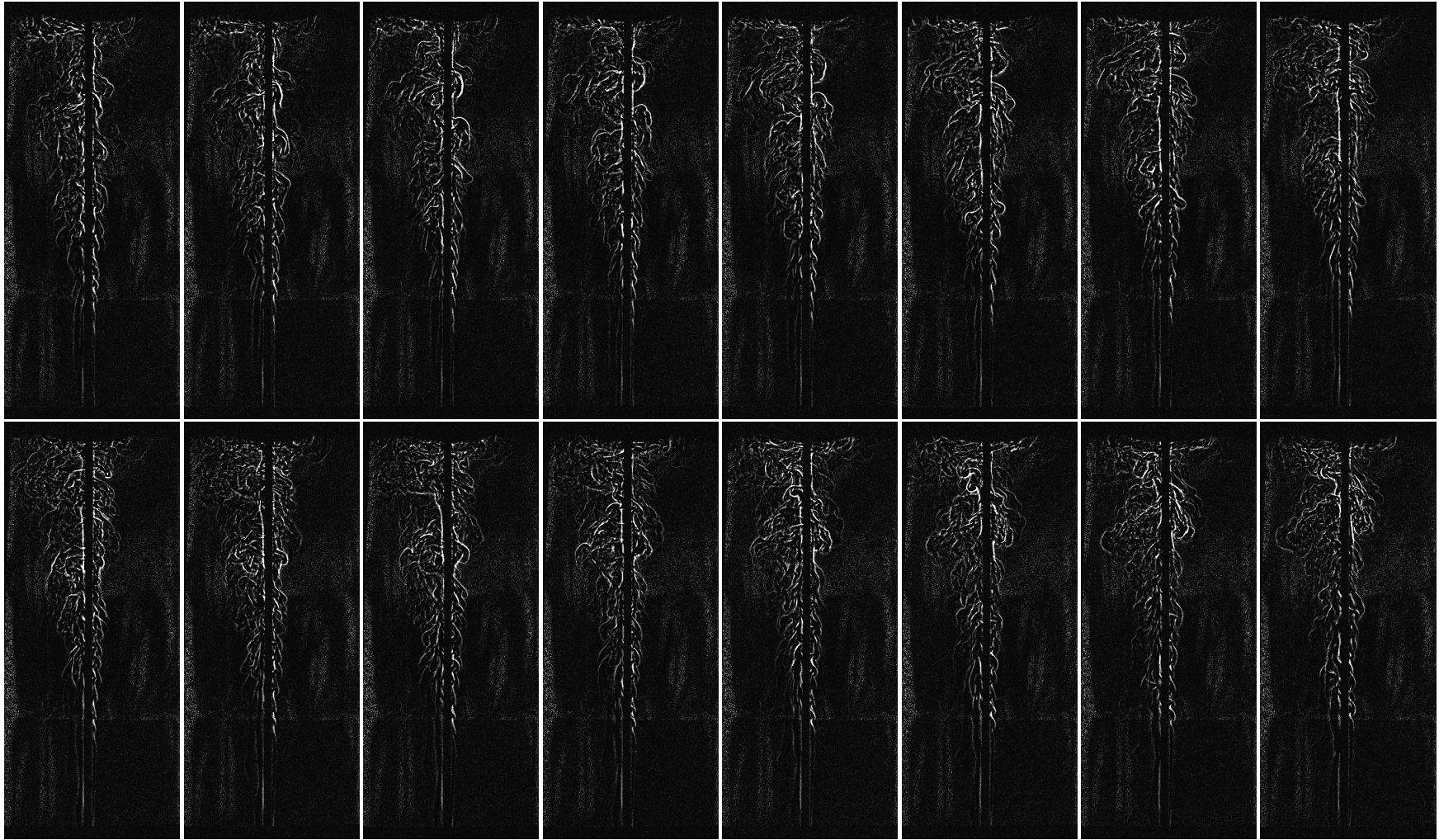
Figure G.4: Processed Shadowgraph image sequence for T_w = 950 K.
