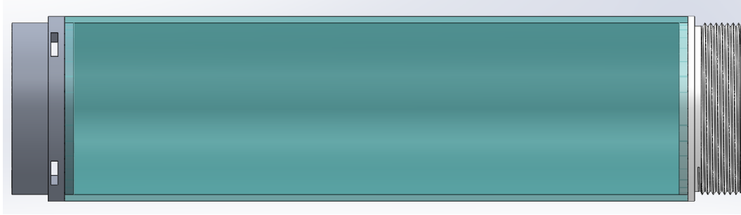
Figure 8: The acrylic housing, in transparent blue, shown around the lips of each end cap.
