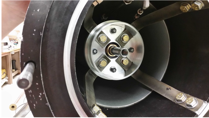
Figure 35: Piston-stopper system installed in the Ludwig tube with the front bumper and stopper removed, showing the tie support connections.
