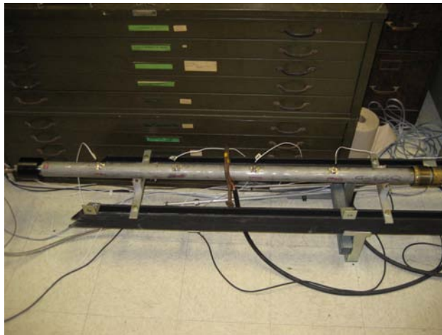
Figure 15: Fully assembled driven section. The large black cable visible is a grounding cable for the driven section to decrease interference from the diaphragm bursting system to the pressure transducers.
