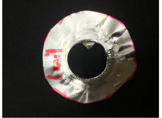
Figure 10: A broken steel diaphragm. Notice that the majority of the center of the diaphragm has been broken and the fragments have been sent down the tube.
