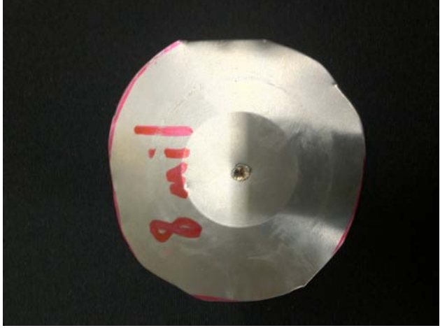
Figure 9: An unbroken aluminum diaphragm. The probe burned a very small hole in the center of the diaphragm, but the pressure difference between sections was unable to force the diaphragm the remainder of the way open.
