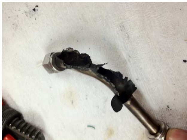
Figure 20: Result of a detonation in the fill line in a similar experiment
