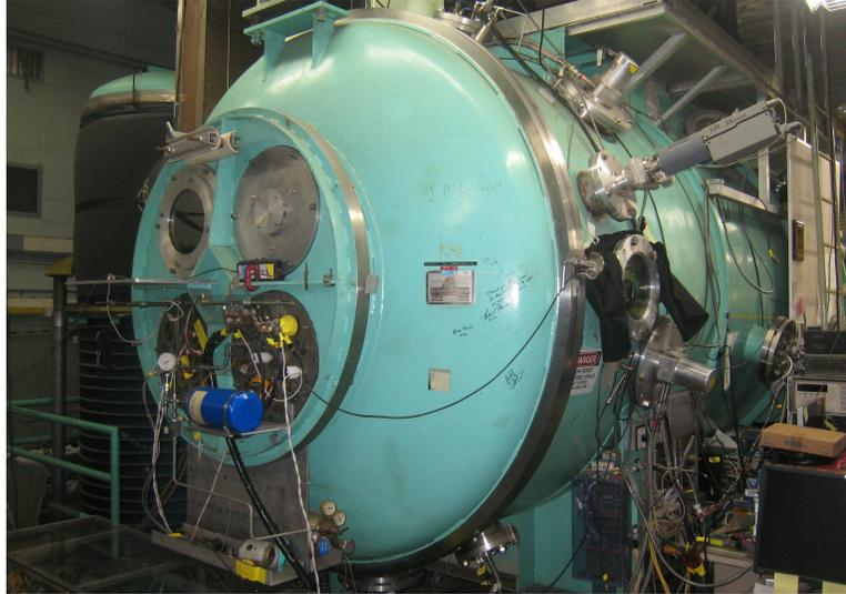
Figure 2.8: Vacuum chamber facility at JPL used for the MPDT experiments.
