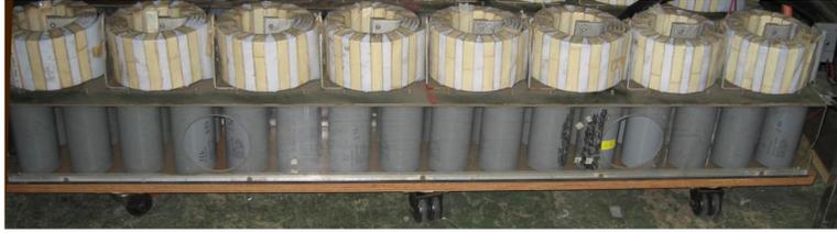
Figure 2.9: Pulse forming network bank.
