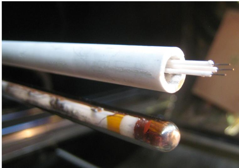
Figure 2.16: Triple Langmuir probe and tungsten wire tips alongside magnetic probe.
