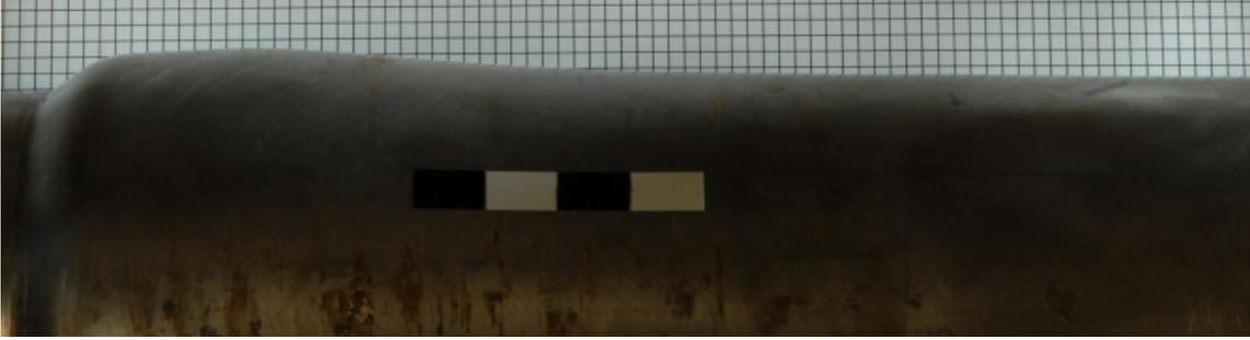
Figure 3.31: Fully deformed tube after 3 detonations at 3 bar initial pressure. Grid spacing is 5 mm.
