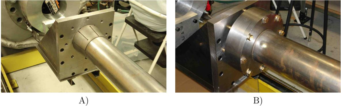
Figure 3.9: A) The collet around the tube prior to installation of the outer ring. B) The final configuration with the tapered retaining ring installed.
