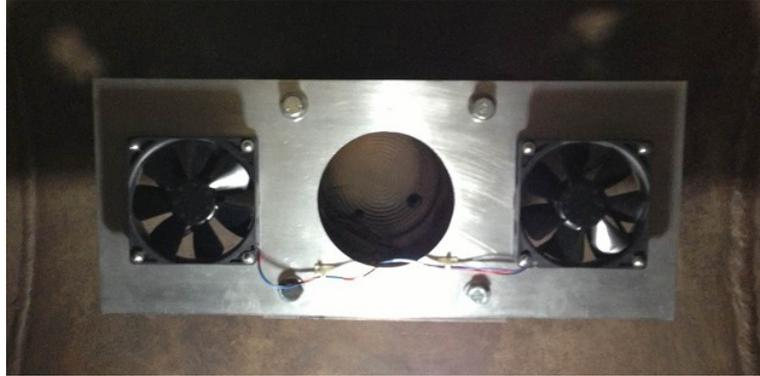
Figure 2.4: Gas premixing tank internal fans.
