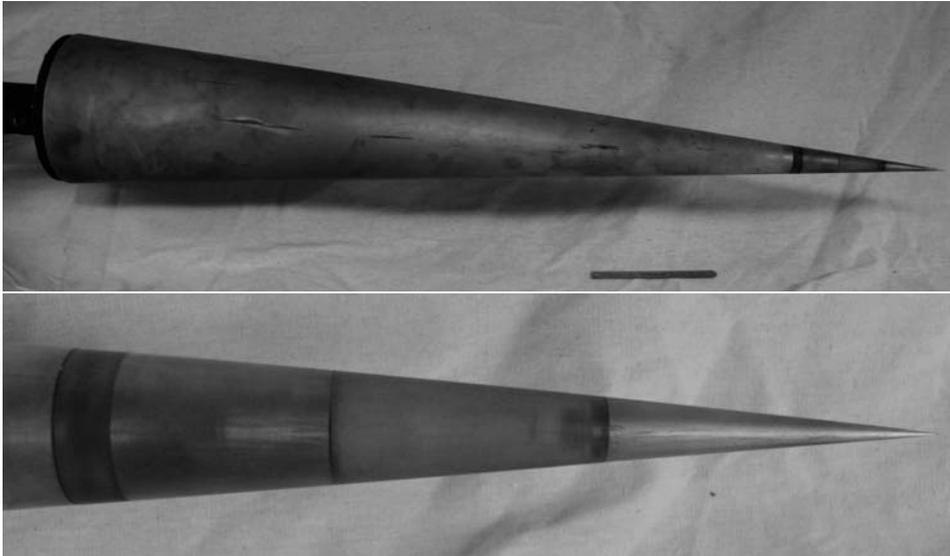
Figure 3.1: Top: Aluminum cone, 1 m in length, instrumented with 80 thermocouples in 20 rows. Bottom, from right to left: molybdenum tip, plastic holder, 316L sintered stainless steel  $10 \mu\text{m}$  porous section, plastic mating section, cone.
