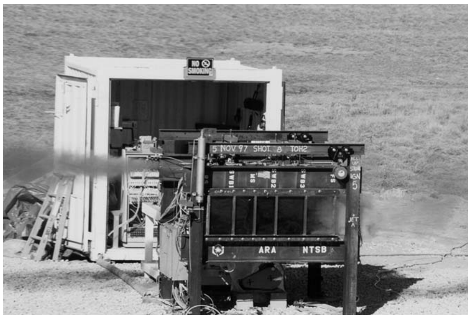
Figure 5.41: Venting of combustion products from vent stringers and leaks in SWB3. The soot acts as a tracer for the flows. Test 8.
