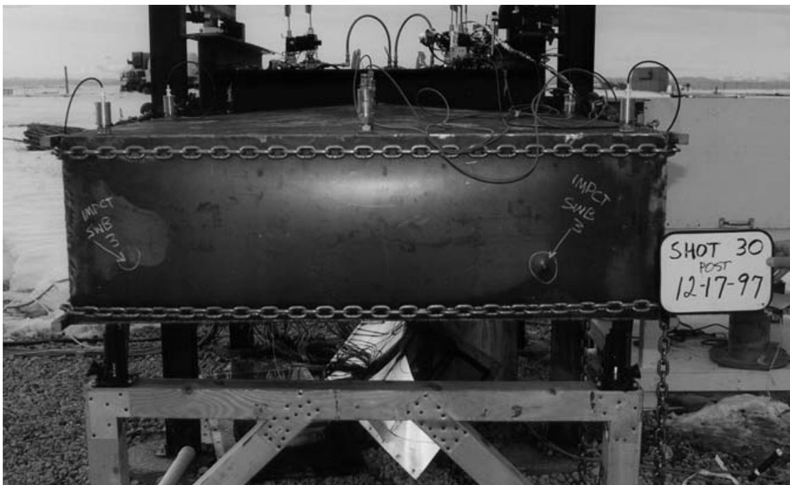
Figure 5.184: End of cargo bay after Test 30. Note that the end plate is bulged, and two dents are present from impact of SWB3. The top and bottom plates of the cargo bay are bulged out approximately 3 in at the centers of the open end.
