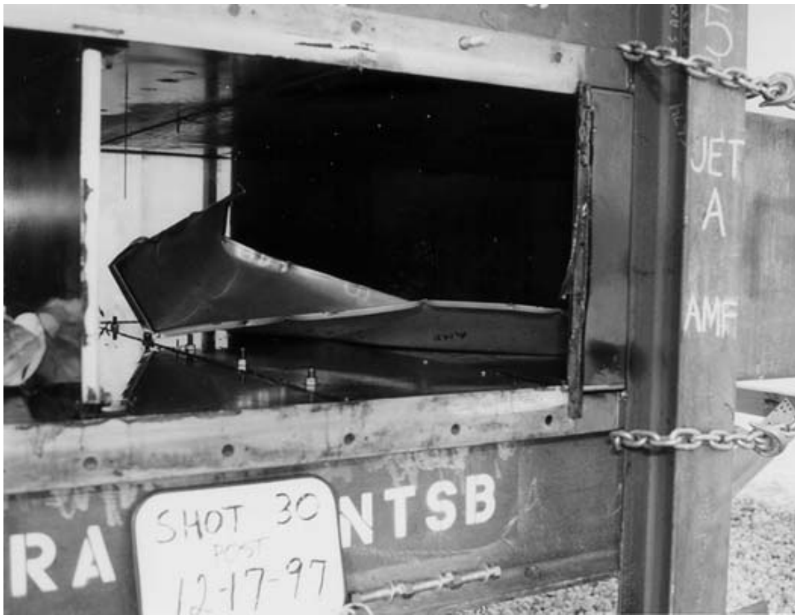
Figure 5.185: Interior of cargo bay after Test 30 (starboard window removed). SWB3 rebounded from the far end and came to rest back in the fuel tank.
