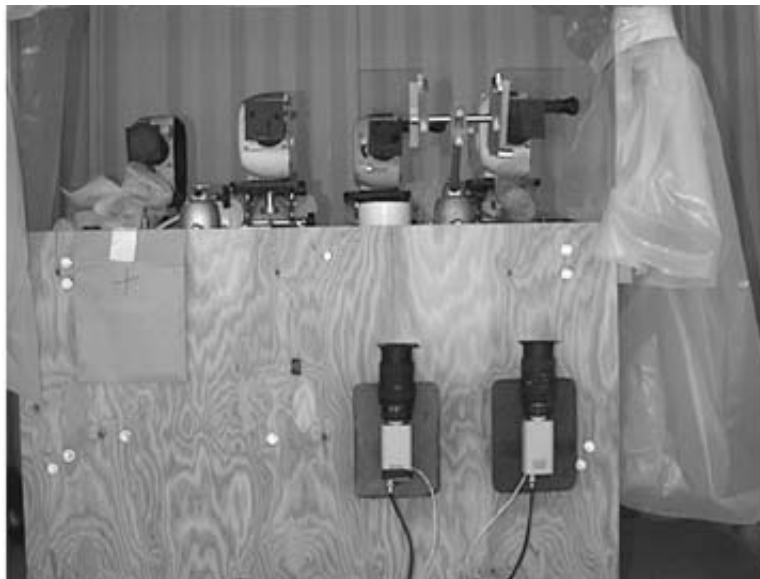
Figure 2.32: High-speed cameras for pseudo-schlieren combustion photography with beam splitters and video cameras.
