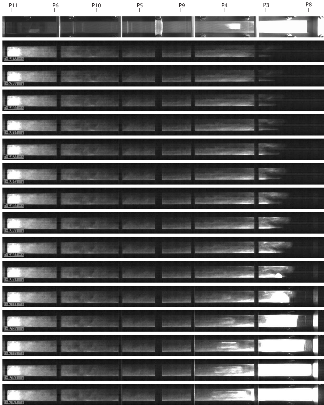
Figure 33: Sequential frames between 5.972 and 6.167 ms from the visualization of shot 15. Time increases from top to bottom. The approximate sensor locations are shown above an image of the test section taken immediately prior to the shot.
