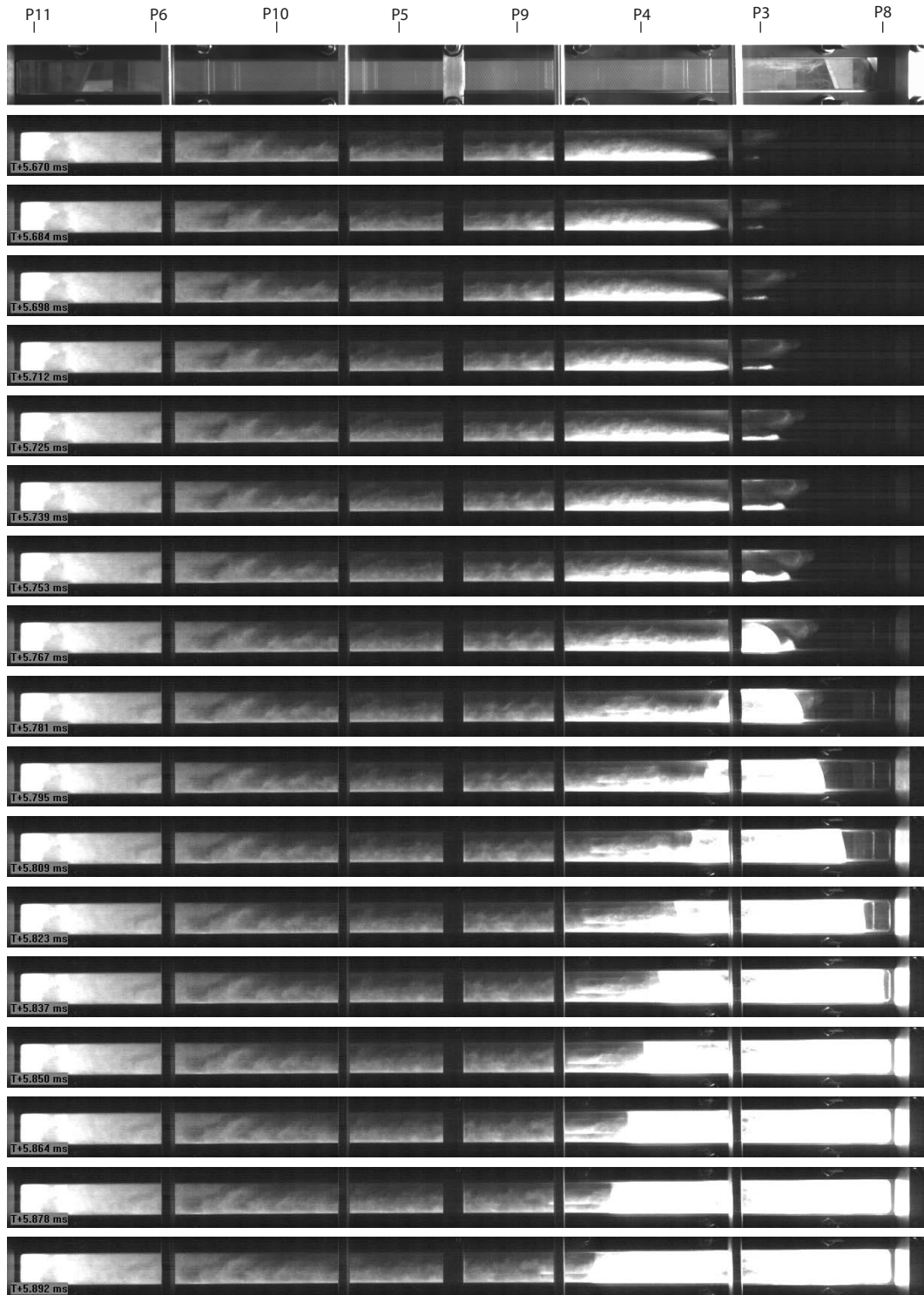
Figure 32: Sequential frames between 5.670 and 5.892 ms from the visualization of shot 14. Time increases from top to bottom. The approximate sensor locations are shown above an image of the test section taken immediately prior to the shot.
