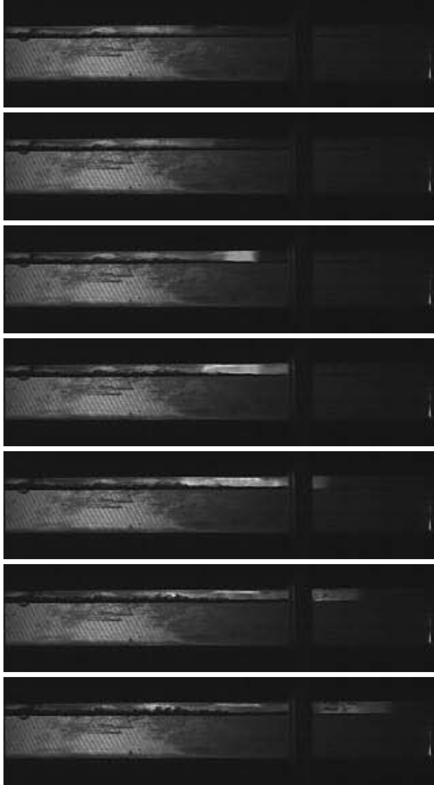
Figure 49: Sequential frames showing enlarged view between 3.219 and 3.455 ms from the visualization of shot 19. The DDT event occurs at about 3.303 to 3.316 ms. Time increases from top to bottom in increments of 13.88 \mu\text{s} . The top image was taken after water filling but prior to ignition.
