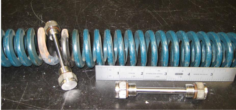
Figure 8: Shchelkin spiral and mounting pins.
