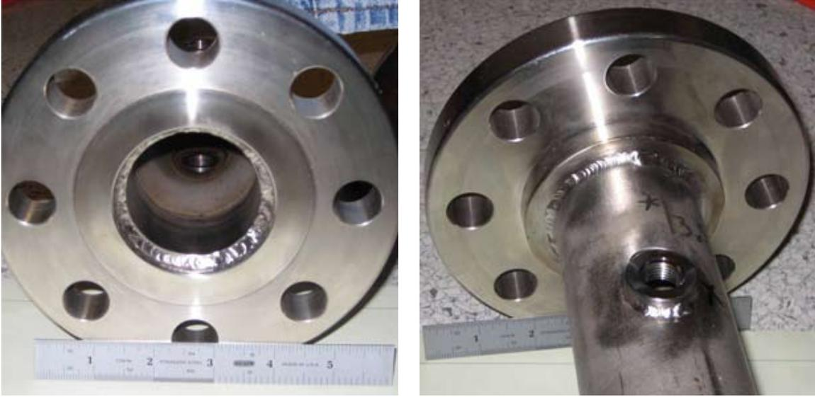
Figure 4: Slip-on flange welds for ES1.
