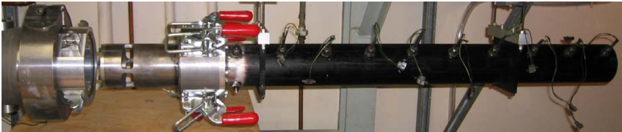
Figure 2. Photograph of annular jet facility showing quick-connect clamps for attachment to shock tube (at left), the annular ports at the left end of the test section, the test section with ion probe gauges and pressure transducers to the right.
