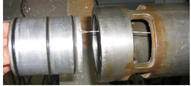
Figure 4. The sliding gate is shown removed from the test section. Note the wire connecting the sliding gate to the pull rod (not shown).
