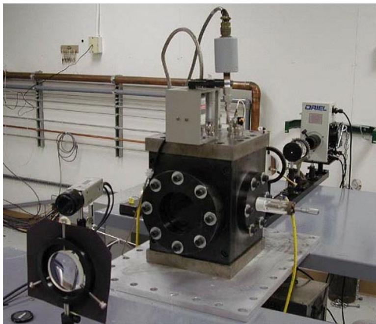
Figure 81: Constant volume combustion vessel for pre-mixed partial oxidation experiments.
