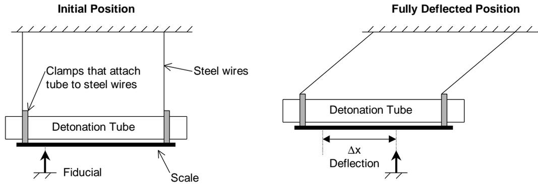
**Figure 1.** Impulse measurement by a ballistic pendulum.
