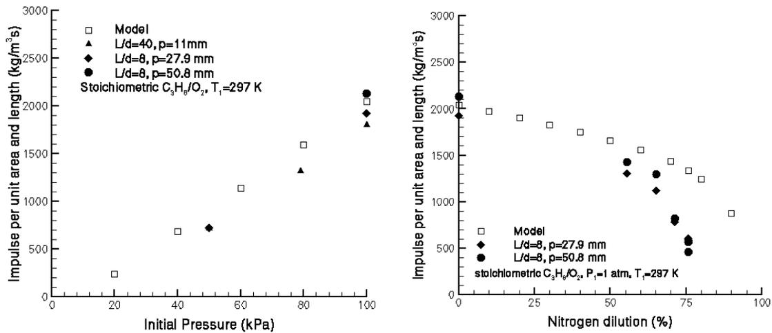
**Figure 6.** Impulse measurements for stoichiometric  $C_3H_8-O_2$  mixtures with varying  $N_2$  dilution and initial pressure for two spiral configurations. Impulse determined from the ballistic pendulum is compared to values calculated from the theoretical model.
