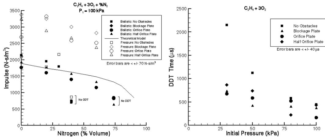
**Figure 8.** Impulse measurements for stoichiometric  $C_2H_4-O_2$  mixtures with varying  $N_2$  dilution and initial pressure for three obstacle configurations. Impulse determined from the ballistic pendulum is compared to values obtained by integrating the thrust wall pressure history and to values calculated from the theoretical model.
