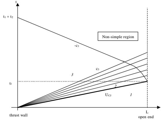
**Figure 3.** Gas dynamic processes inside the detonation tube.
