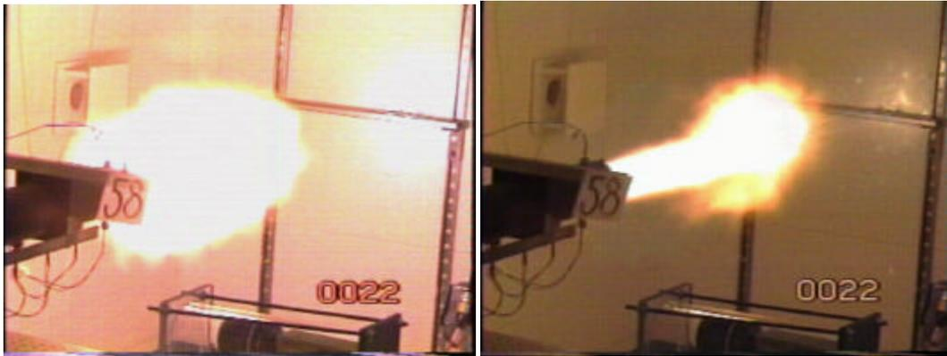
**Figure 5.** Combustion products expanding out from a detonation tube. The initial mixture was  $2C_2H_4+6O_2+2N_2$  at 100kPa.
