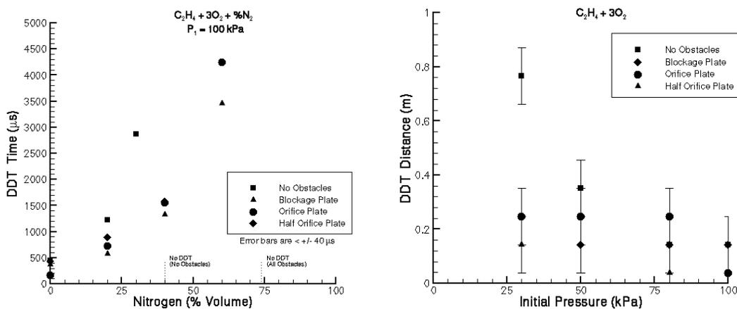
**Figure 7.** Measured DDT time for stoichiometric  $C_2H_4-O_2$  mixtures with varying  $N_2$  dilution and initial pressure for three obstacle configurations.
