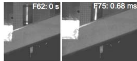
Figure 14 - Impactor penetrating into the target in Test 7 with no deformation of outer surface in 0.8 ms.
