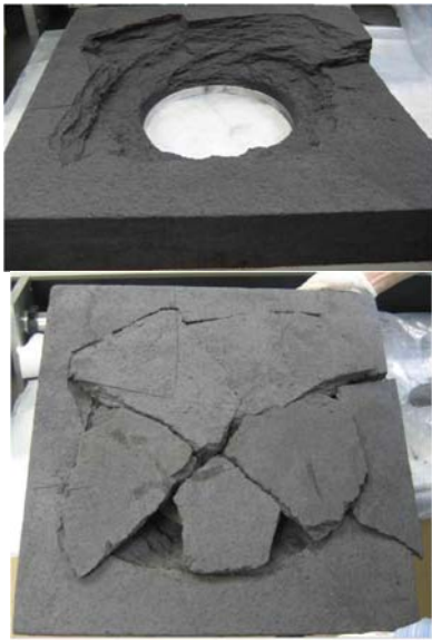
Figure 12 - The Fiberform® target after impact during test 6: 1) the port in the target created by the impact on the push plate, 2) the target reconstructed from the fragments of Fiberform® blown out from the impact.
