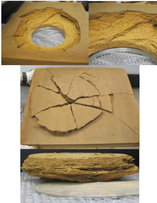
Figure 17 - PICA target impact damage during Test 8.
