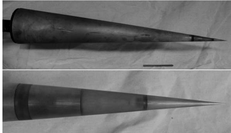
Figure 1. Top: Aluminum cone, 1m in length, instrumented with 80 thermocouples in 20 rows. Bottom, from right to left: molybdenum tip, plastic holder with 316L stainless steel 10 micron porous section, aluminum cone body.
