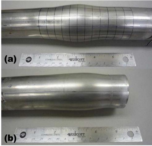
Figure 14. Post-test photographs of specimen bulges for shot 103, short tube,  $V_B = 71.4$  m/s: (a) near the buffer bottom; (b) near the specimen bottom end.
