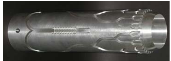
Figure 5: The second generation toroidal initiator. The outer sleeve has not yet been placed over the inner sleeve in this view.
