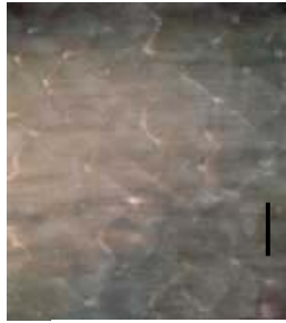
Figure 2: Soot foil of JP10-20% C_2H_2 -Air. Detonation propagated from left to right.
