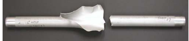
Figure 13: Crack propagation and bifurcation under detonation loading. Detonation propagated from left to right. P_{CJ}=6.2 MPa, notch length 50.8 mm.
