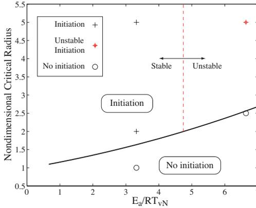
Fig. 5. Critical radius based on the critical decay-rate model as a function of  $E_a/RT_{vN}$ .
