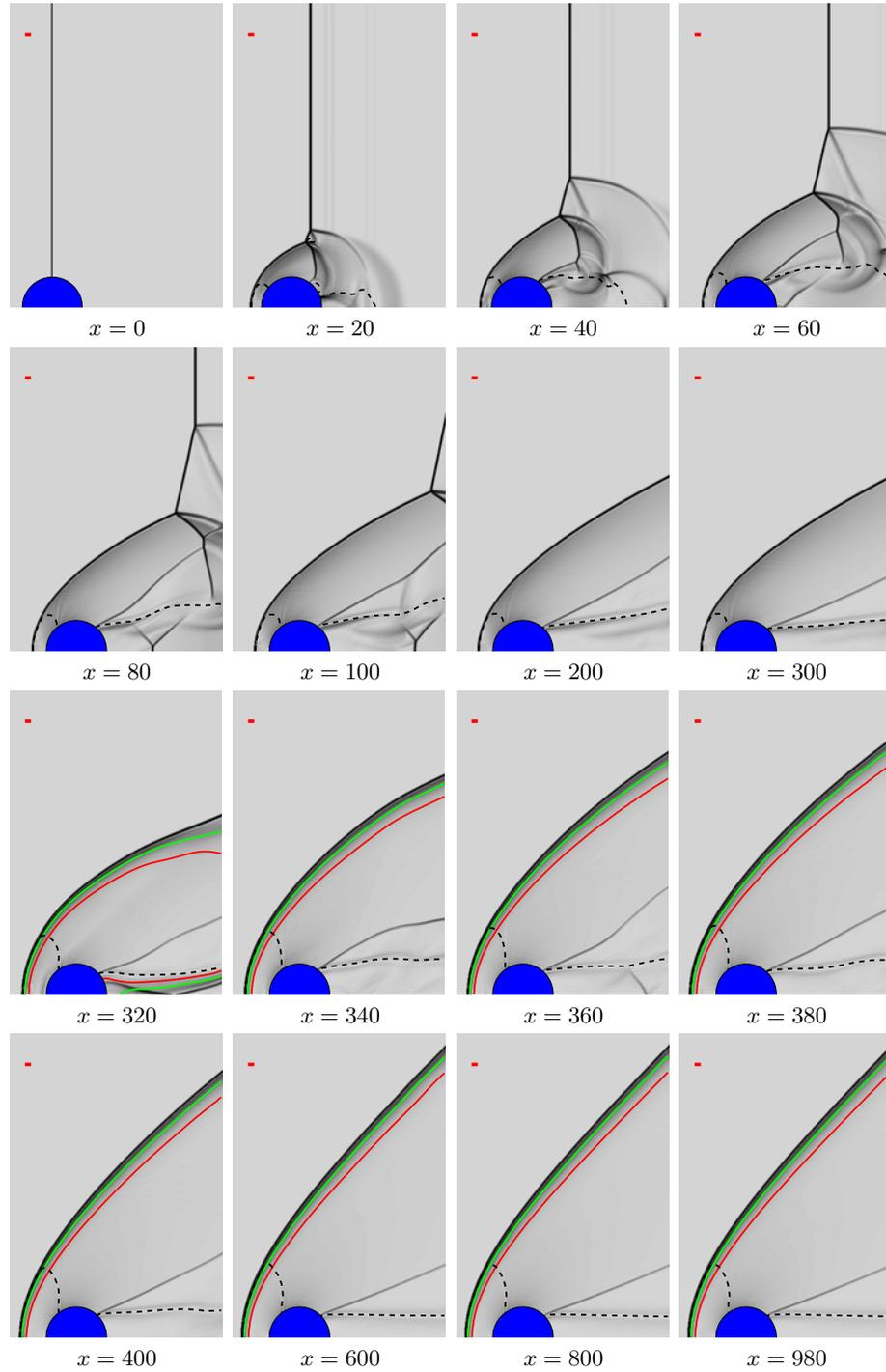
**Fig. 2.** Numerical Schlieren and reaction contours for case b16. The black dashed line is the sonic locus.
