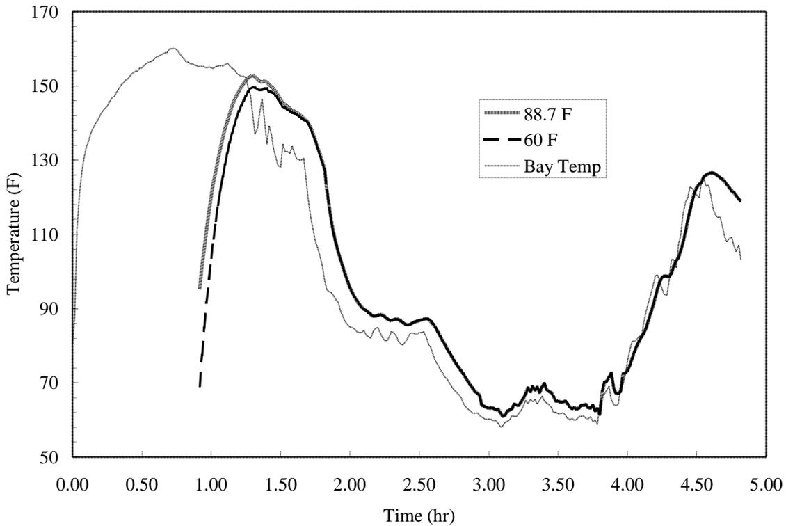
**Figure 10:** Estimated effect of initial fuel temperature, flight 6 ACM bay conditions. Fuel mass of 300 lb, corresponding to estimated amount in TWA Flight 800.
