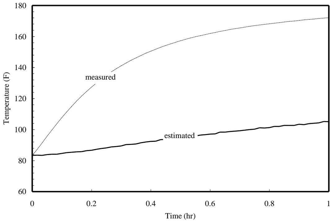
**Figure 11:** Comparison of measured and estimated fuel temperatures for the initial ground portion of flight 1. 50 gallons of fuel (300lbs). The  $hA$  used in the calculation is 400W/K, obtained from the flight 6 calibration.
