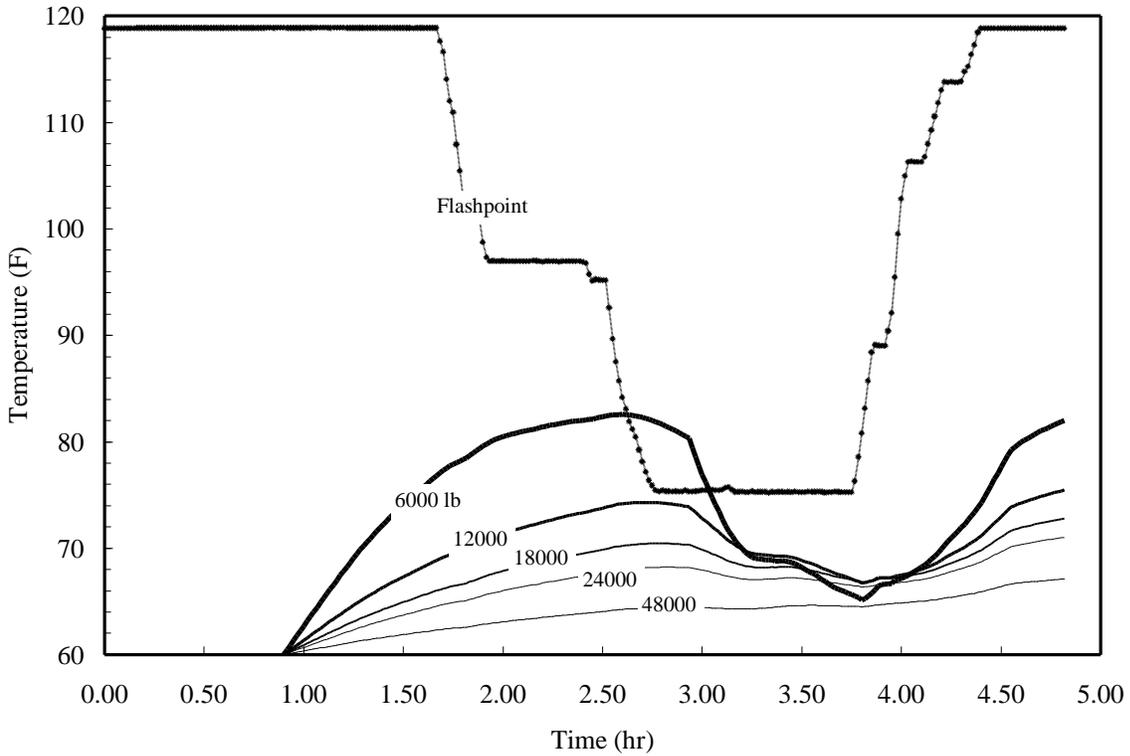
**Figure 9:** Estimated effect of added fuel mass variation, flight 6 ACM bay conditions. Fuel initial temperature of 60 F.
