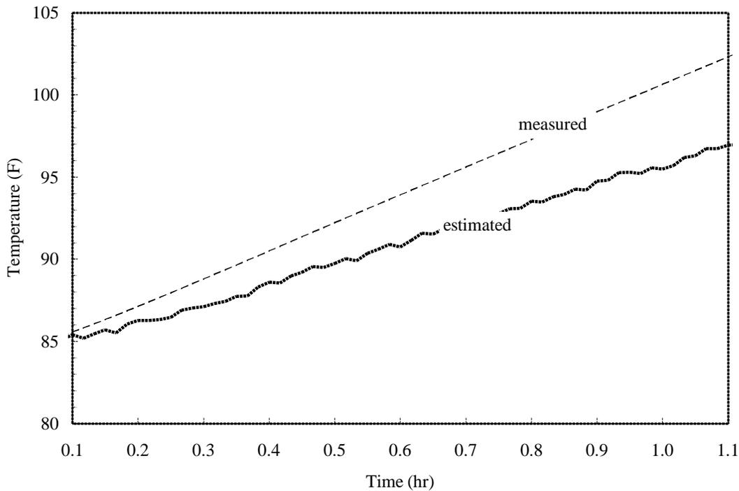
**Figure 12:** Comparison of measured and estimated fuel temperatures for the initial ground portion of flight 5 with 6000 lb of fuel. The  $hA$  used in the calculation is 400W/K, obtained from the flight 6 calibration.
