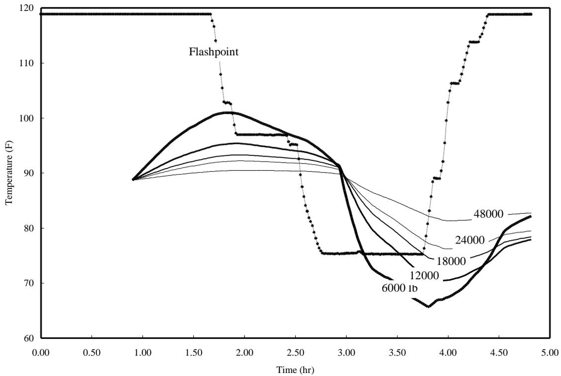
**Figure 6:** Estimated effect of added fuel mass variation, flight 6 ACM bay conditions. The initial fuel temperature at the beginning of the calculation was 88.7 F, which is taken from the measured fuel temperature in the tank at that time point.
