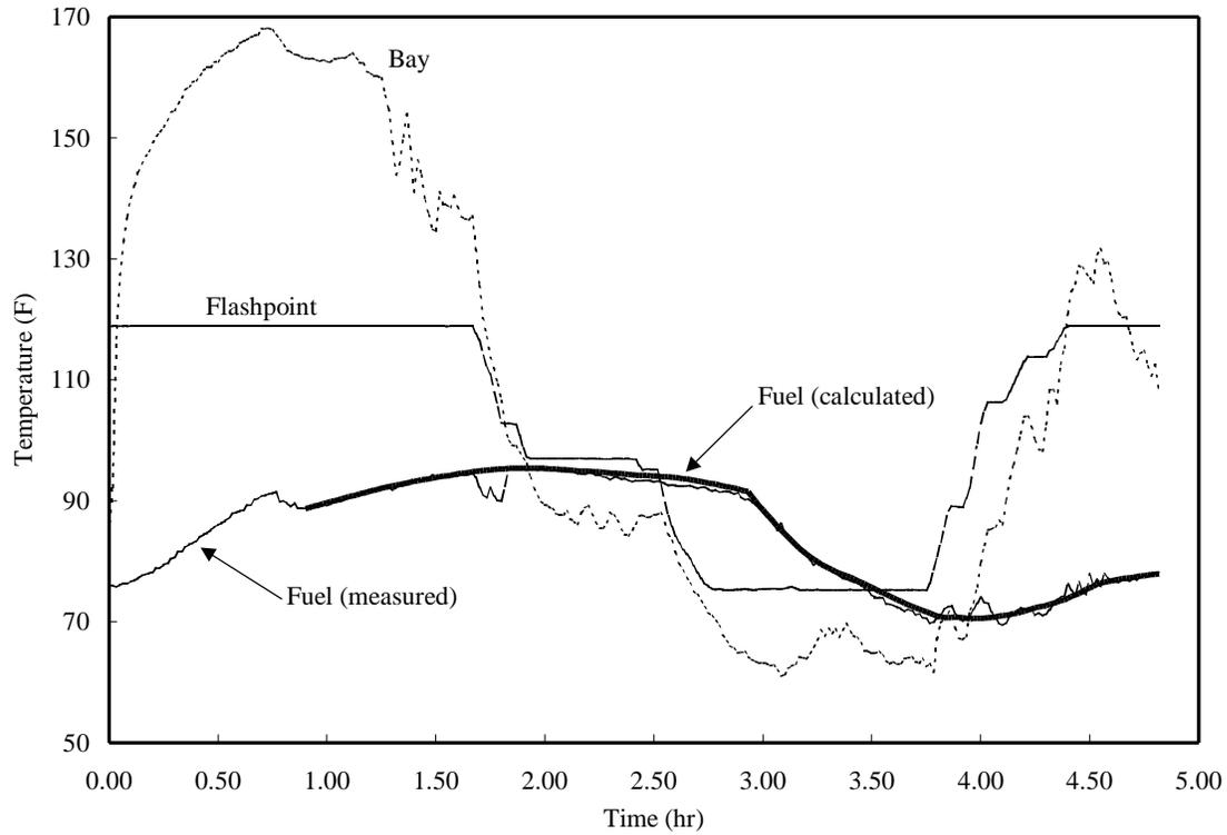
**Figure 3:** The calculated temperature of the 12000 lb of fuel in flight 6, calibrated with measured data.
