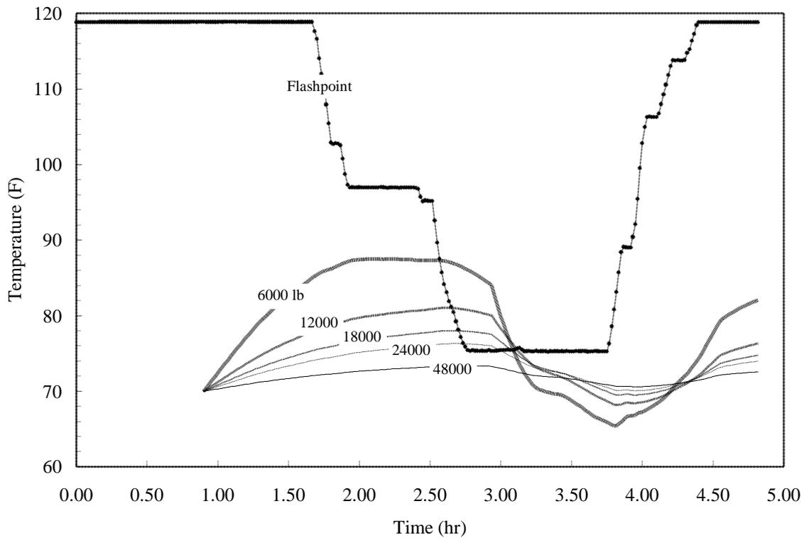
**Figure 8:** Estimated effect of added fuel mass variation, flight 6 ACM bay conditions. Fuel initial temperature of 70 F.
