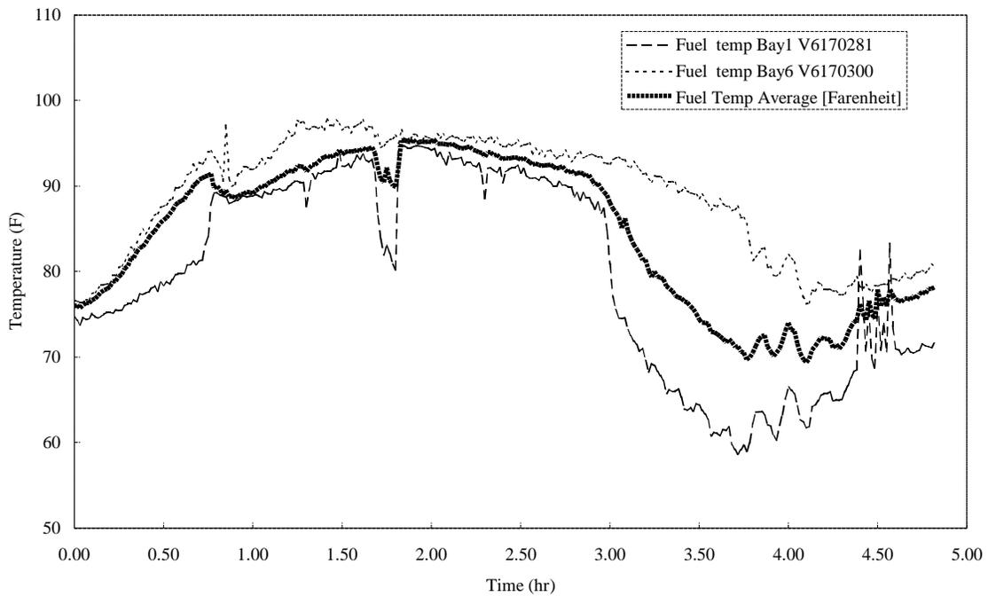
**Figure 2:** The measured temperatures in the fuel tank. The thermocouples were located within a few inches of the bottom of the CWT.
