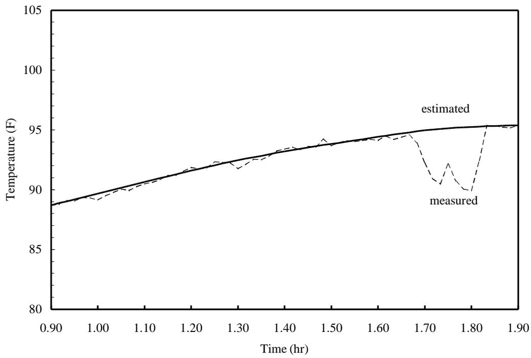
**Figure 13:** Comparison of measured and estimated temperatures for initial ground portion of flight 6. The value of  $hA$  used in this portion of the calculation is  $400\text{W/K}$ .
