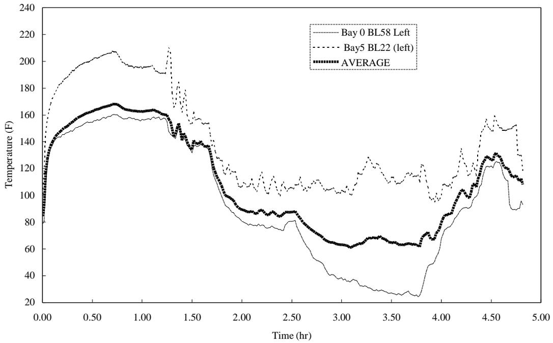
**Figure 1:** The maximum, minimum and average (over 20 traces) of measured temperatures in the ACM bay. The thermocouples were located 4 inches below the bottom of the tank.
