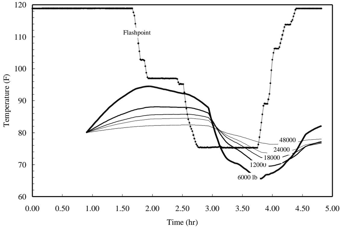
**Figure 7:** Estimated effect of added fuel mass variation, flight 6 ACM bay conditions. Initial fuel temperature of 80 F.
